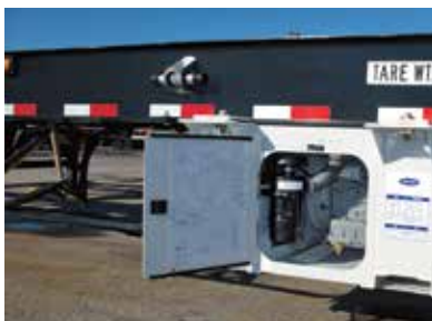
Large service opening improves access, reduces service time while on chassis.
